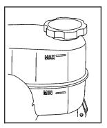
Look at the brake fluid reservoir. The fluid level should be above MIN. If it is not, have your brake system checked to see if there is a leak.
